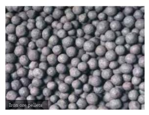
improved performance of the kiln. The use of iron ore pellets reduces loss on ignition. Two of the different iron ore pelletization processes are (i) straight travelling grate process and (ii) grate kiln process.
