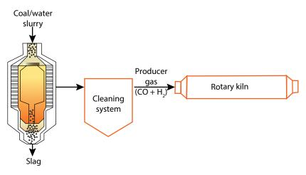
Coal gasification system for rotary kiln in sponge iron production
