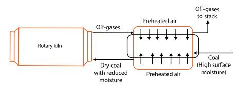
WHR-based rotary drum dryer for surface moisture removal for coal
