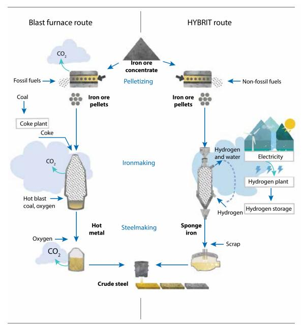
Comparison of blast furnace route and HYBRIT route *Source: HYBRIT*
