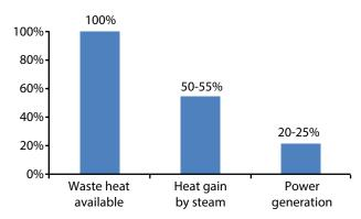
Waste utilization from rotary kiln
