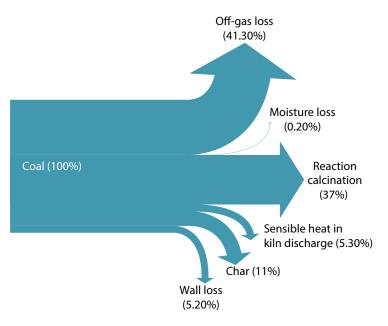
Typical energy balance of a coal-based rotary kiln
